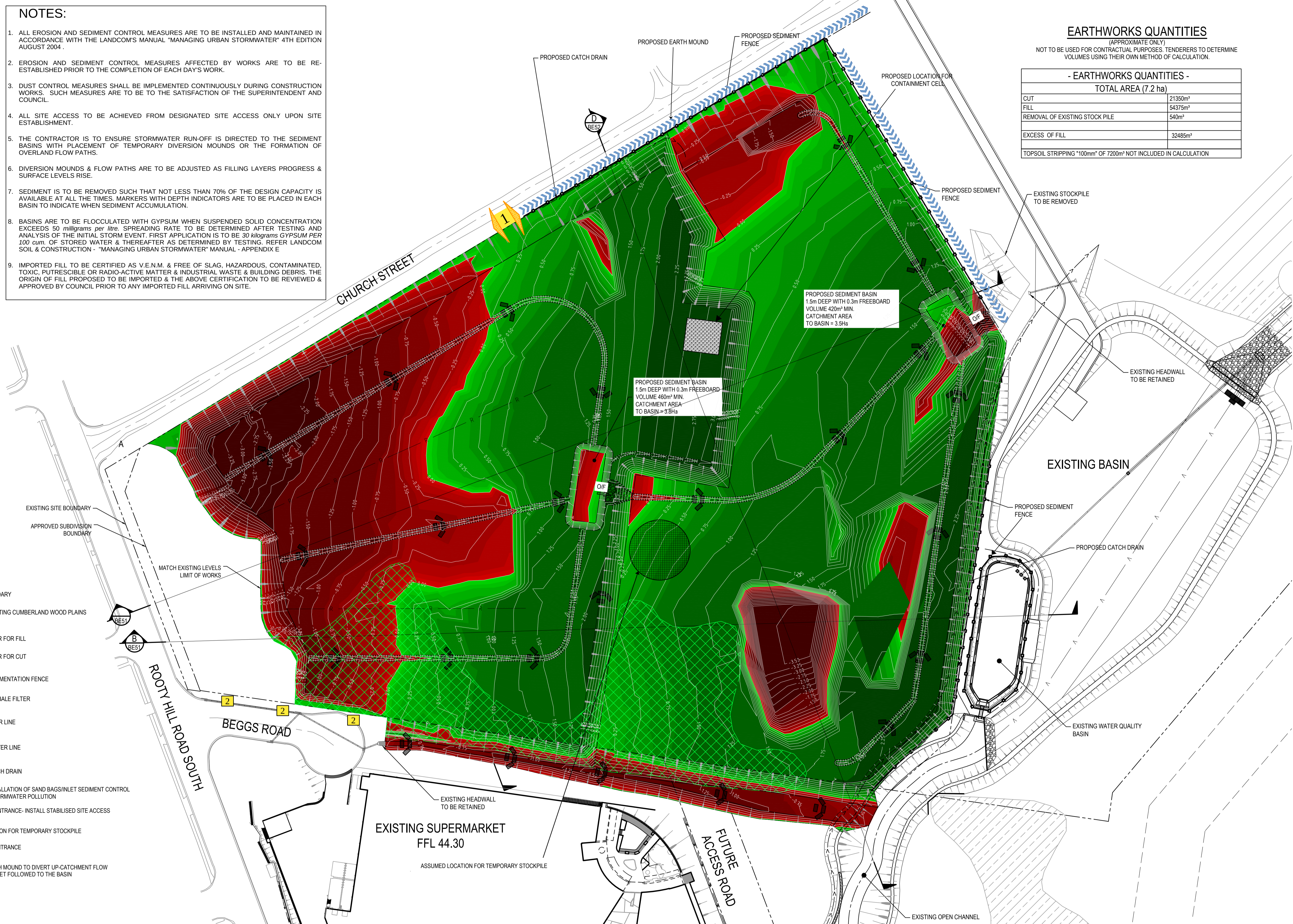
EARLY WORKS - CUT AND FILL PLAN
